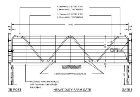
The frame shall be of tubing of bore 42 mm and wall thickness of 2,0 mm in the case of main frame members, and of a bore 22 mm and wall thickness of 2,0 mm in the case of bracing members. The width of each gate shall be as shown on the drawings.
