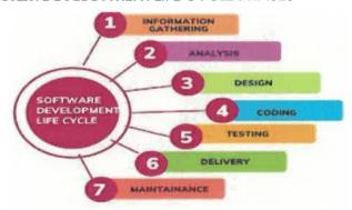
The DRDAR's SDLC policy includes seven phases, during which defined work products and documents are created, reviewed, refined, and approved. Not every project will require that the phases be subsequently executed and may be tailored to accommodate the unique aspects of a project. These phases are described in more detail in the following paragraphs.
